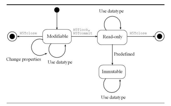
Figure 24. Transient datatype states: modifiable, read-only, and immutable
