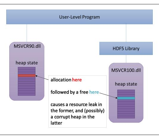
Figure 1. How the heap corruption and resource leaks might occur
