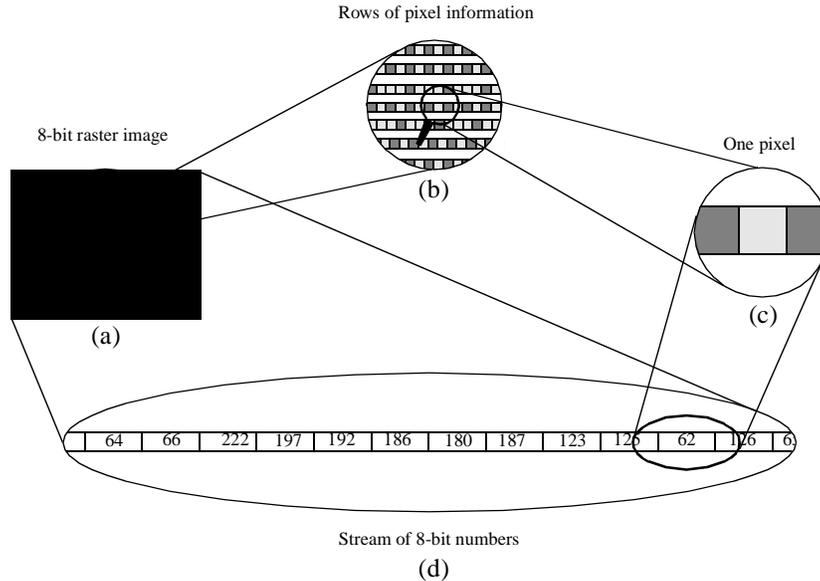
**An 8-bit raster image (a) is a set of rows displayed from left-to-right consisting of rows of pixel information (b) where each pixel (c) is represented by values stored as a single stream of 8-bit numbers (d).**
