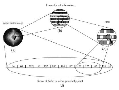
A 24-bit raster image (a) is a set of rows displayed from left-to-right consisting of rows of pixels (b) whose values are stored as three 8-bit numbers (c) in a stream of data (d). In this figure, the image is interleaved by pixel.
