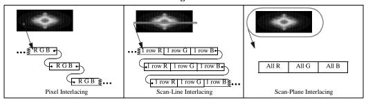
An interlace format describes both the physical format of an image as it is stored in memory and in the file. When writing to a file, HDF stores a 24-bit image using the same interlace format as it has in memory. However, when reading from a file, it is possible to make the in-core interlacing mode different from that used in the file. The following table contains a summary of the interlacing format available in the DF24 interface.
