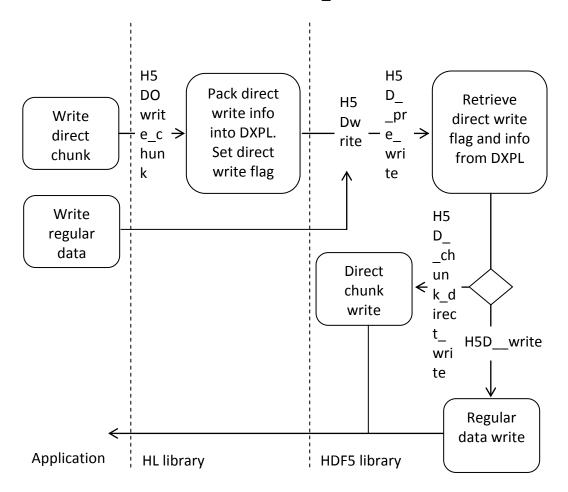
Figure 3. Diagram for H5DOwrite\_chunk in the high-level library
