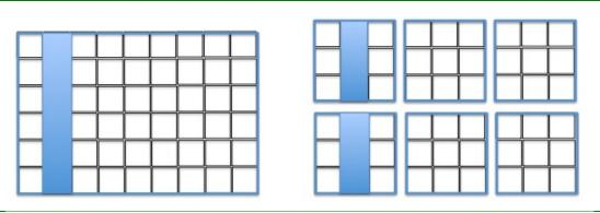
Figure 9: Each chunk is stored separately in the HDF5 file. Two chunks will be read by HDF5 to access the 2nd column of the array.
