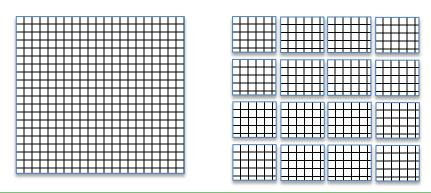
Figure 1: Data array is logically split into equally sized chunks each of which is stored separately in the file.
