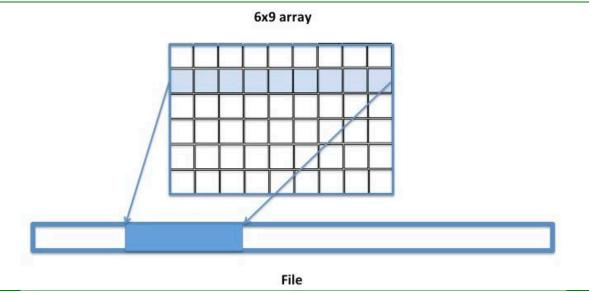
Figure 7: Elements of the rows of the 6x9 two-dimensional array are stored contiguously in the file while elements of the columns are not.
