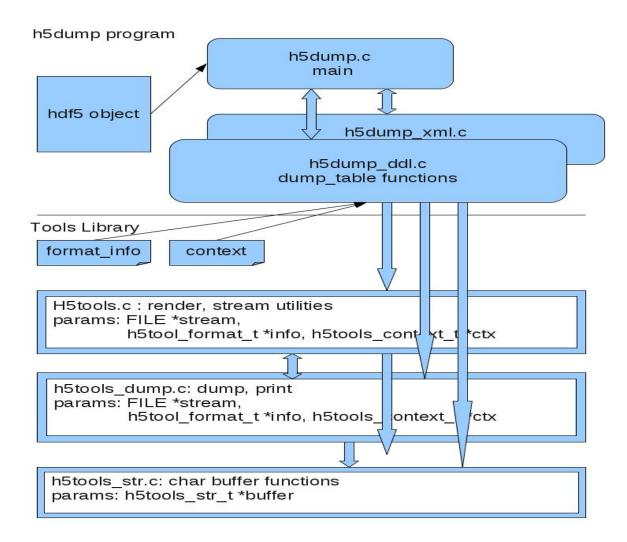
**Figure 2 Refactored Code Layout**
